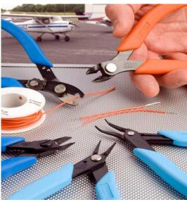
the Model 505ST adjustable stripper for stranded wire down to 26 gauge without nicked wire strands.
